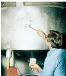
Stainless Steel Putty is ideal for making non-rusting repairs to stainless steel food processing equipment.
