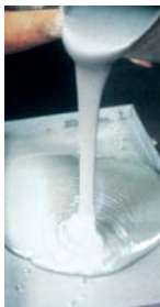
Aluminium Liquid is a low-viscosity, pourable epoxy for making molds, patterns and holding fixtures.
