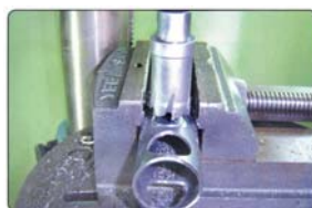
Stainless steel pipe boring
