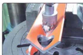
Angled steel boring
