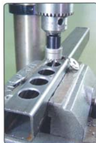
Square pipe boring
