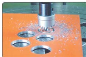
Steel plate boring
